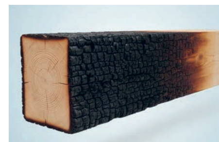
Illustration of the char layer on a fire test beam
